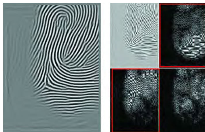
Figure 2. On the left an enhanced fingerprint, on the right its one-level decomposition by Haar wavelet (the selected bands are highlighted).
