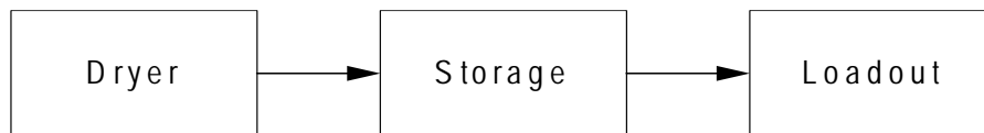
Figure 2. Simplified Flowchart of Current DDGS Processing Steps that Could be Augmented by Value-Added Processing.
