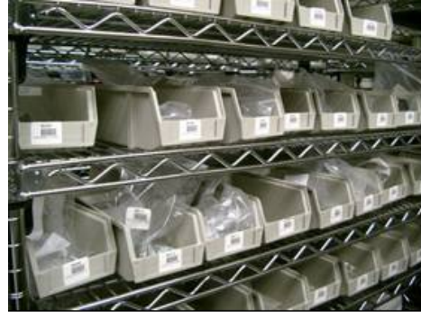
Plate 4: Bar coded storage bins used on the rolling storage racks
